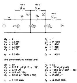
tune  $L_2$ ,  $C_2$  for an attenuation peak at  $f_1$  tune  $L_4$ ,  $C_4$  for an attenuation peak at  $f_2$
